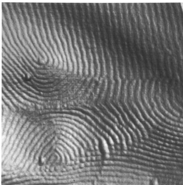
Figure 2: Atomic force microscopy image of a diblock copolymer of poly(styrene- block -butadiene). The length of the figure is 2.1 \mu\text{m} .
