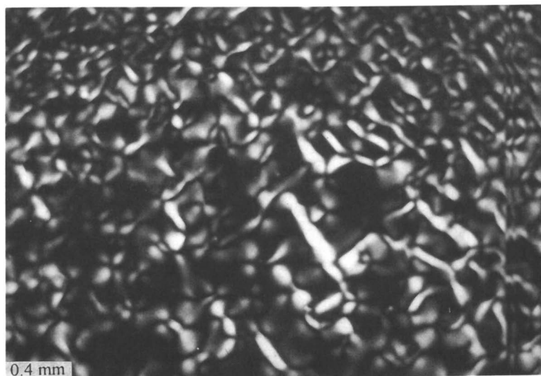
Figure 2. Photomicrography of the Texture of PA-1 formed in the process of solvent evaporation.
